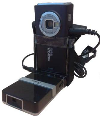
**Figure 2: A N95 mobile phone and a PK101 projector assembled to a wearable gadget**
