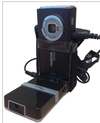
**figure 1.** Our prototype: A mobile phone and a micro projector assembled to a wearable gadget
