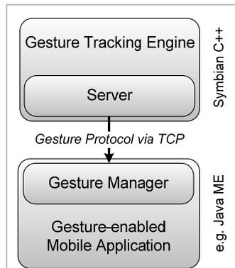
**figure 2.** Simplified architecture of the gesture detection framework
