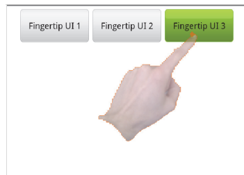
Figure 9. Segmented hand mask blended into user interface
