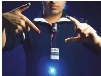
Figure 3. 6th Sense uses colored markers to ease fingertip detection
