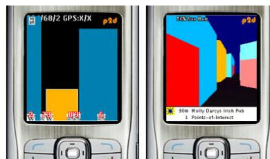
Figure 2: 2D billboard model (left) and 3D block model (right)
