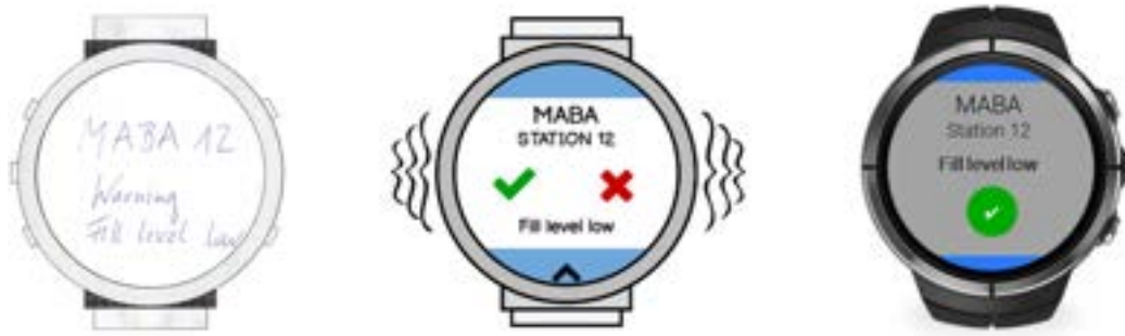
Figure 2: One example of the iterative co-creation of a wearable monitoring app from sketches (left) over wireframes (middle) to a functional prototype for a Wear OS-powered smartwatch (right).
