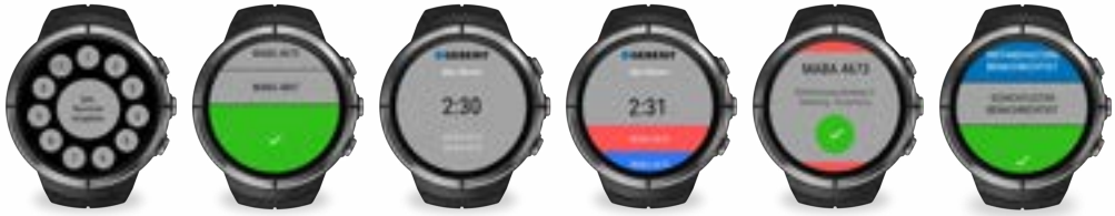
Fig. 3. The core screens of the monitoring app for smartwatches: login with employer ID, machine selection, main screen with time display and machines registered, an unsolved warning and error, detail screen of an error, and the selection of the measure taken (from left to right).
